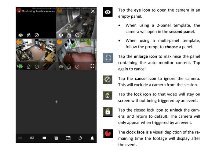
This button toggles between large and small video panels within the auto monitor.
