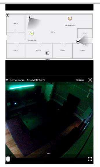
In the example alongside, the camera associated with the output is displayed beneath the map.
